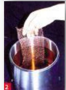
**NB.** If sediment is added to the distiller the mix is liable to foam on heating and overflow creating a hazard. The sediment can give your spirit an unpleasant sour aroma and flavour. If in doubt add a few drops of Distilling Stabiliser to the liquid before switching the unit on.
